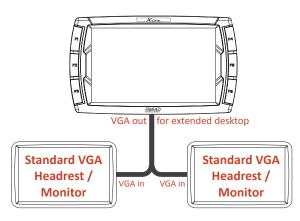
VGA Output compatible with market headrest monitor for passengers information media (PIM) with independent content from driver mobile data terminal
