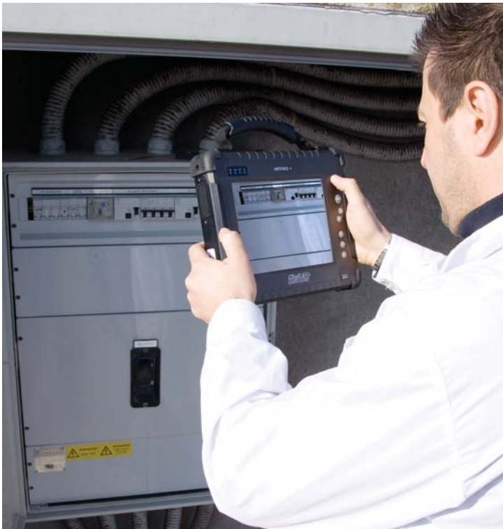
NITRO+ Tablet PC with embedded 1.3Mp camera, HSUPA modem, GPS receiver with antennas, allowing outdoor live geo-referenced video/picture streaming
