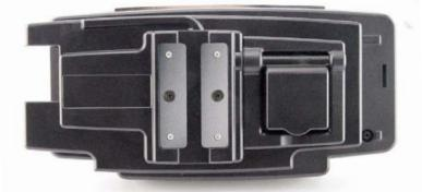
Antennas connectors, for eventual easy antenna swap from indoor to outdoor antennas, in case of weak signals, due to extremely shielded windscreen glass.
